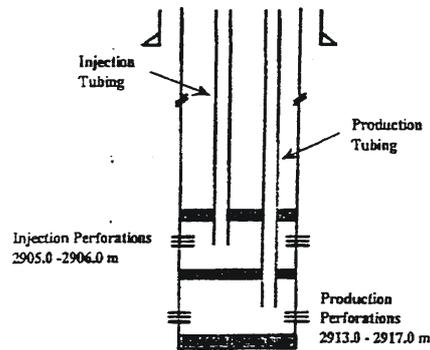
**Figure 3:** schematic of well completion, the approach: inject the oil again. Also in schematic figure, well head equipment to inject again is represented. Produced oil from well passes a divider and part of this oil is separated and used to inject again.
