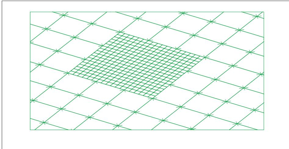
Figure 10: XY view of grid with used LGR around one of the wells:
