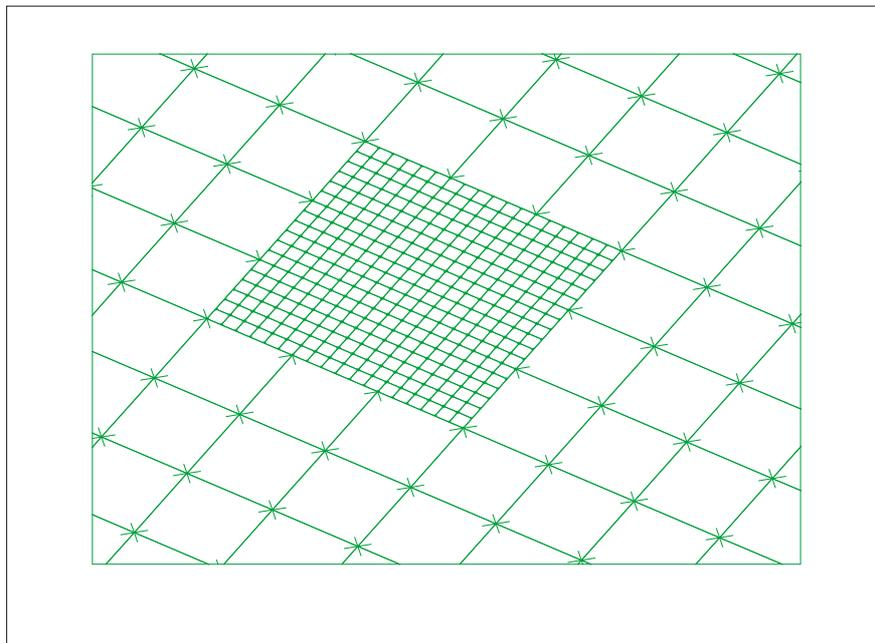
Figure 9: XY view of grid with used LGR around one of the wells
