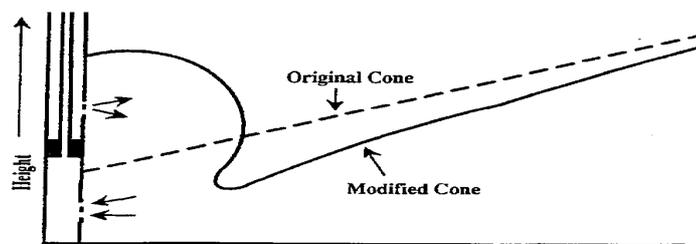
Figure 2: schematic of a cross-section of near region to well spout with/without oil injection
