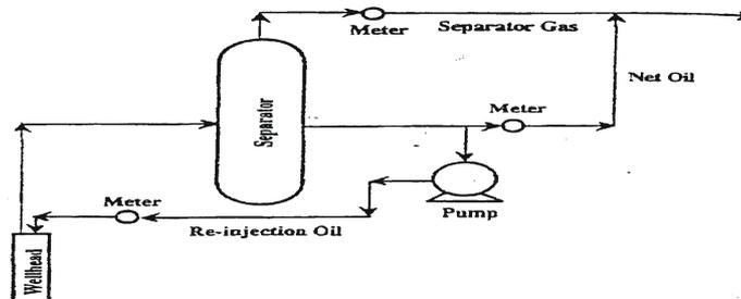
**Figure 4:** schematic of well head equipment to inject the oil again. Injection of chemical materials for reduction of relative permeability of water and gas. Use of chemical materials like gels, foams, polymers and washer materials for injection in water or gas region for reduction of relative permeability can be used in this approach.
