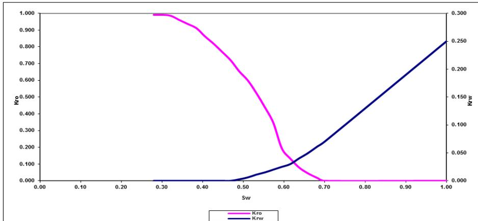
**Figure 11:** curve of relative permeability for one of the oil layers of reservoir
