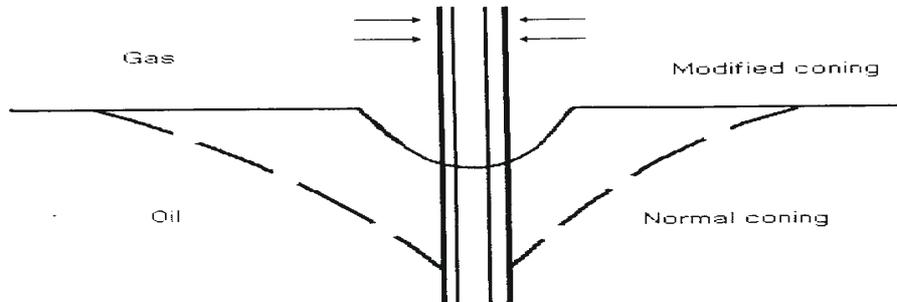
Figure 6: schematic of creation of additional holes in watery or gas region.
