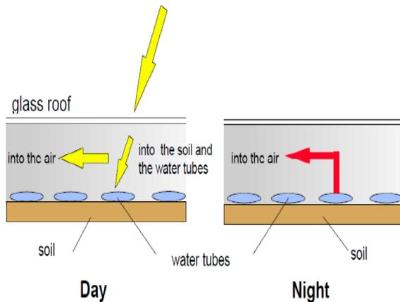
**Fig.7.**principle of storage underneath the roof using water-filled black tube
