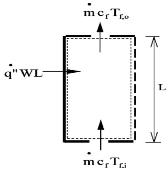
**Fig.5.**Heat balance to air stream in direction of flow For a short length of wall ( $L$ ), the temperature of the glass ( $T_g$ ) and the wall ( $T_w$ ) may be assumed constant and the useful heat transferred to the air flowing in the gap is given by
