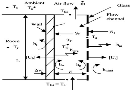
**Fig.3.**physical model of solar chimney
