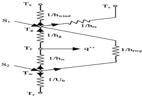
**Fig.4.**Thermal network for solar chimney
