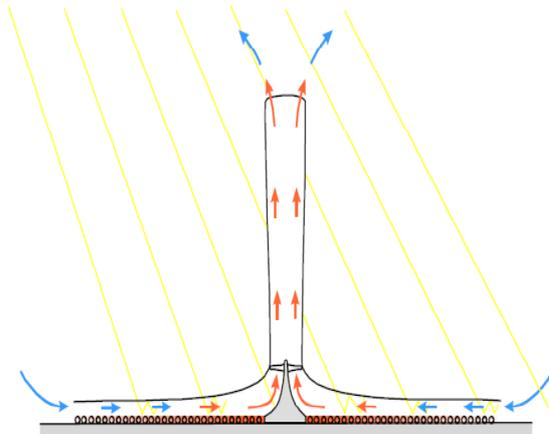
Fig.6. Active solar chimney
