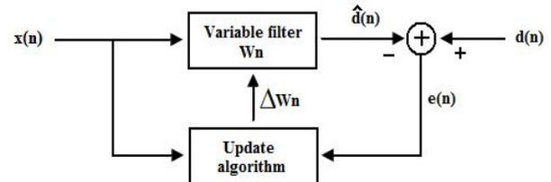
**Figure 3:** A general block diagram of adaptive filter
