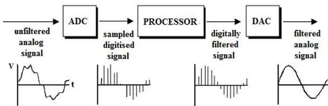
**Figure 2:** A block diagram of a digital filter
