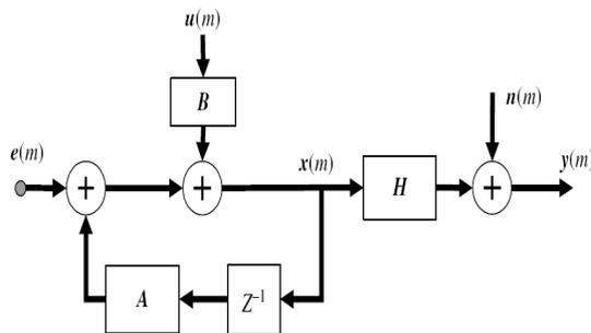
Figure 4: A block diagram of Kalman filter
