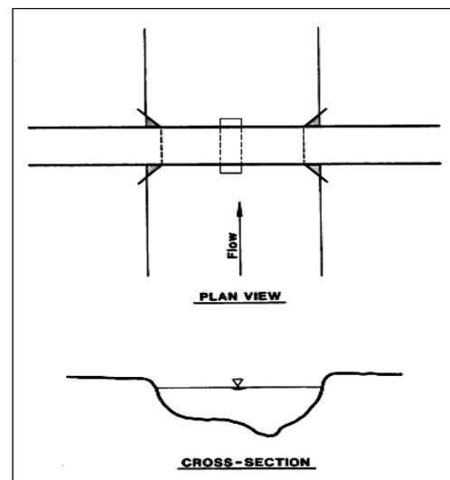
**Fig1.** Scour due to flow narrowing section (FHWA, 2001)
