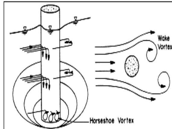
**Fig2.** The mechanisms of candles foundation local scour (Richardson, 2001)
