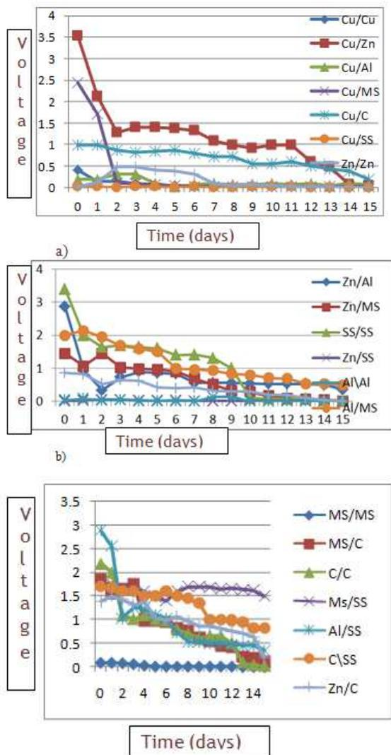
**Fig 3:** the above figures (a, b, & c) shows comparison of voltage (mv) generated by different combination of electrodes.
