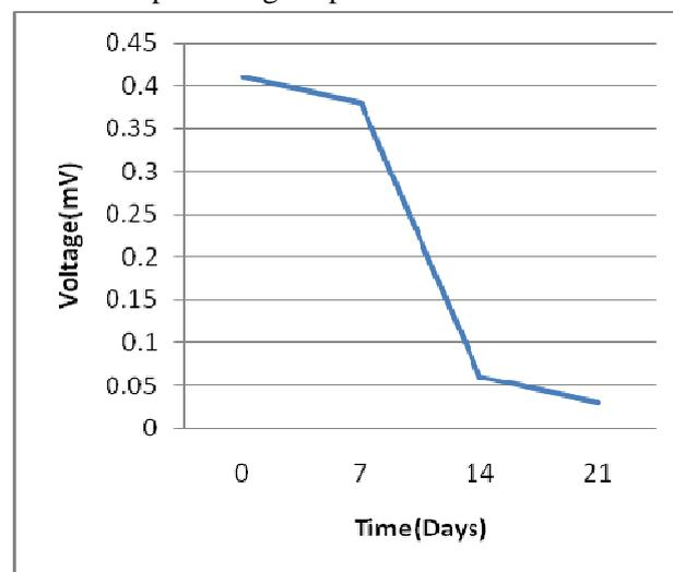
Fig 2: voltage generated using cowdung as a substrate
