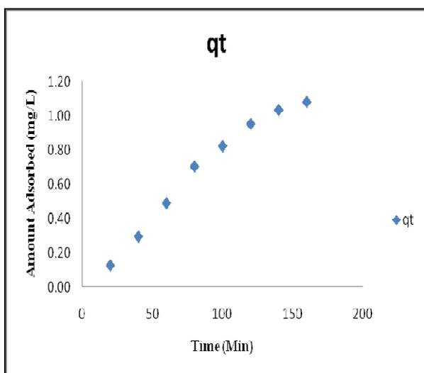
**Fig 2:** Effect of contact time on adsorption of dye solution (CR) on fly ash based activated carbon at Co- 50 mg/l & adsorbent dosage- 30mg/l
