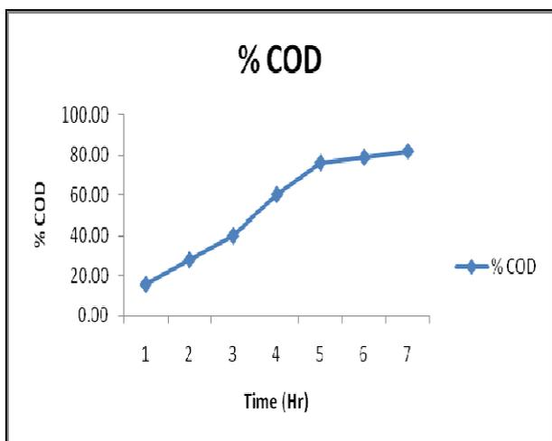
**Fig 9:** COD Removal by the BC from MB containing dye solution
