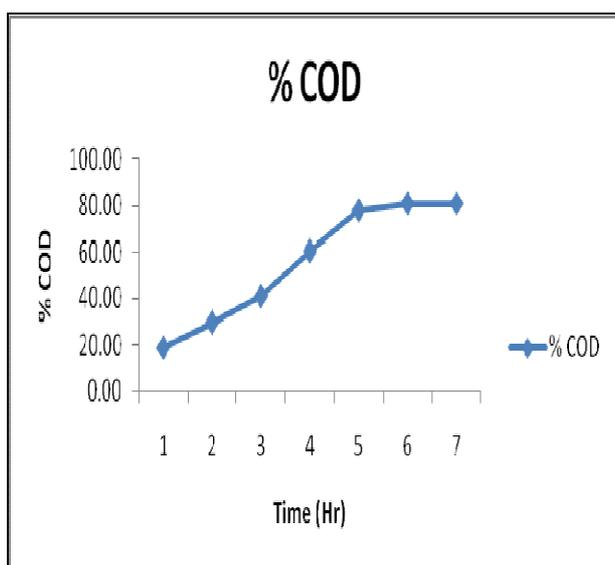
**Fig 10:** COD Removal by the BC from CR containing dye solution
