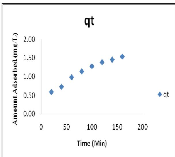
**Fig 1:** Effect of contact time on adsorption of dye solution (MB) on fly ash based activated carbon at Co- 50 mg/l & adsorbent dosage- 30mg/l
