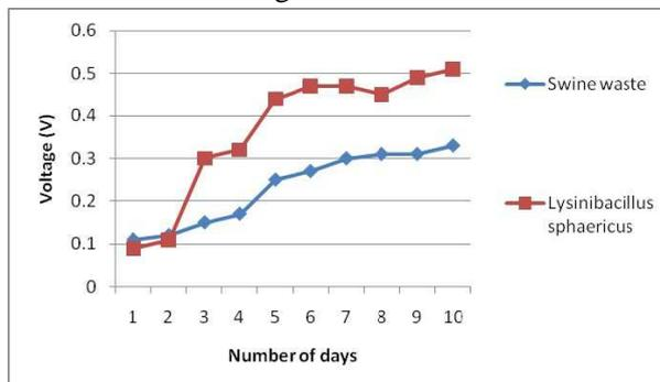
Figure 2: Voltage production of swine waste and *Lysinibacillus sphaericus* DMS-3
