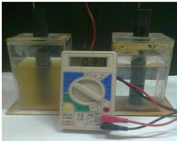
Figure 1: MFC developed with swine waste in anode chamber
