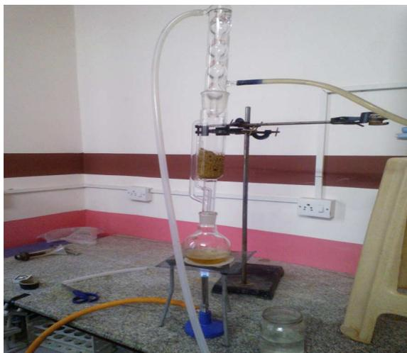
**Fig: 1.** Extraction of dried leaves and Flower using soxhlet apparatus
