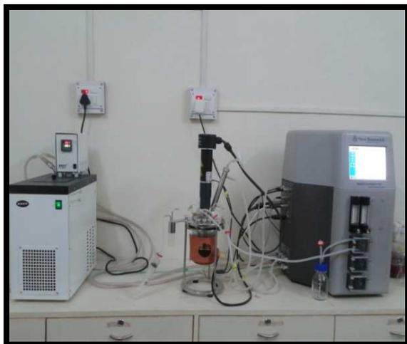
Fig. 2(a) Lab scale fermenter
