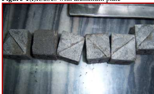
Figure-1(ii). Cubes with cracks
