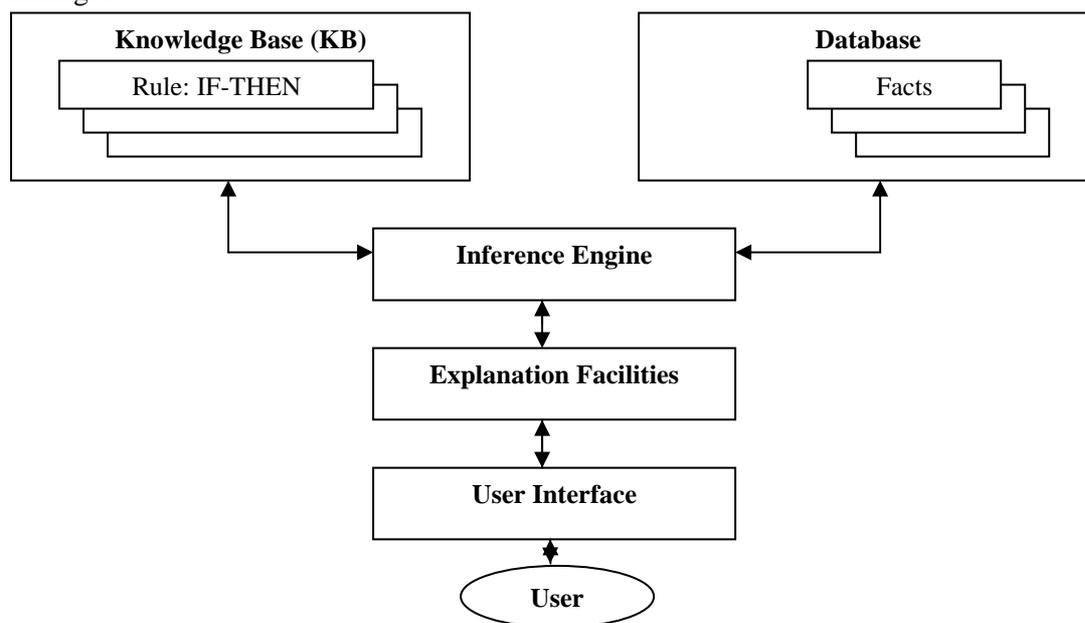
**Fig.1** Components of Expert System and User interface
