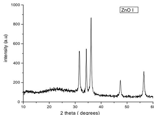
Fig: 1(b). XRD pattern of synthesized nano ZnO
