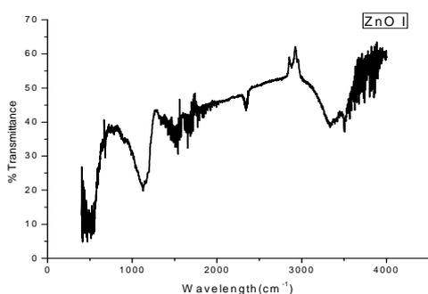
Fig: 2(b). FTIR spectrum of synthesized nano ZnO
