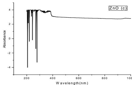
Fig: 3(a). UV- visible Spectra of commercial ZnO
