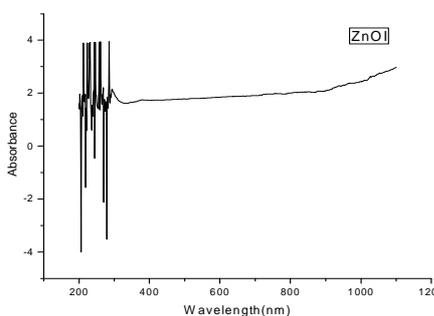
Fig: 3(b). UV- visible Spectra of synthesized nano ZnO
