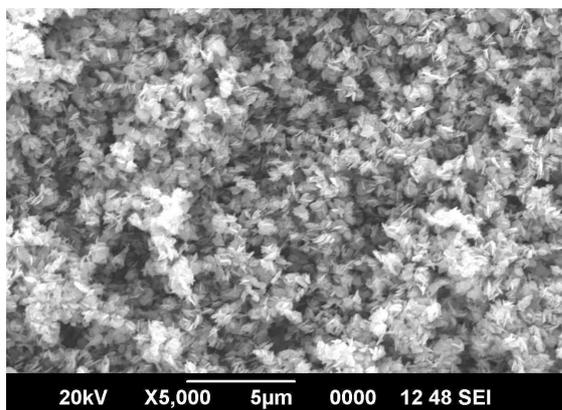
Fig: 4(b). SEM of synthesized nano ZnO
