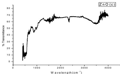
Fig: 2(a). FTIR spectrum of commercial ZnO
