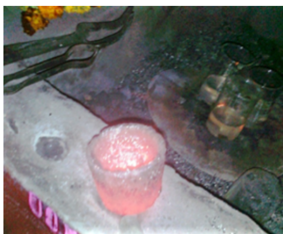
Fig. 7. Smelting Process for Silver Recovery with Continuous addition of Ammonium Chloride for removing the impurities and for getting the white color to the silver.
