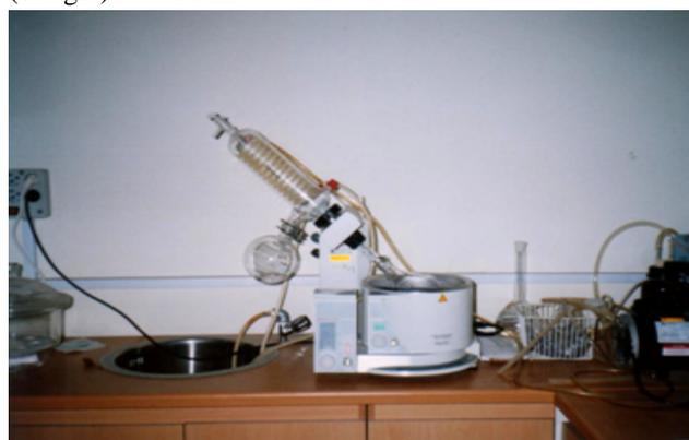
**Fig 2.** Isolation method of fatty acid in Canola seed (Sarigol) from additional solvent, n-hexane with evaporator rotor.
