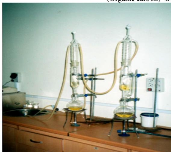
**Fig 1.** Extraction method of fatty acid of Canola seed (Sarigol) with soxhlet
