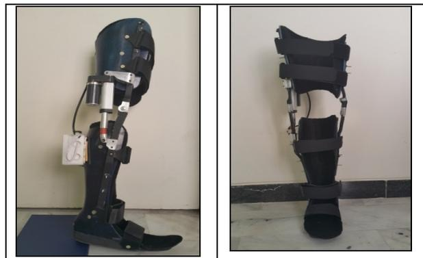
**Figure1:** stance Control KAFO (side view and front view)
