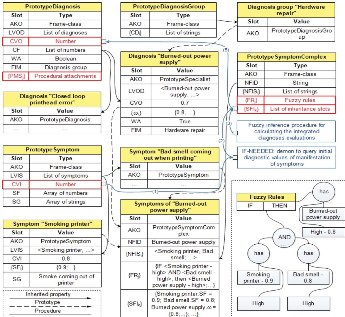
Figure 2 –Knowledge representation for printer diagnosis using the hybrid knowledge base
