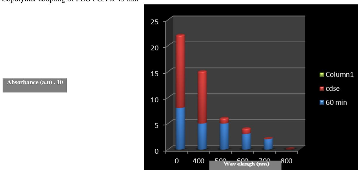
**FIGURE 4.** Absorption spectrum CdSe QDs and the solution containing quantum dots of cadmium selenide with Copolymer coupling of PEG PCA at 60 min
