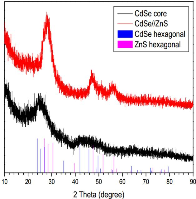
**Figure 1.** XRD patterns of CdSe QDs & ZnS NPs
