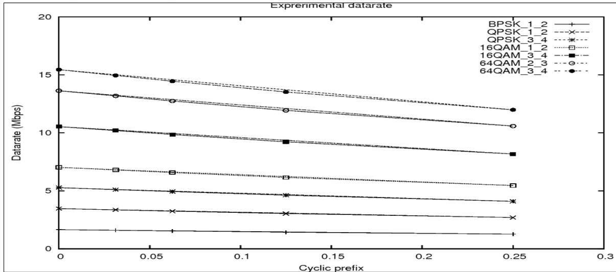
Fig 2: Graph of cyclic prefix vs. data rate.
