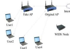
Fig.1. Structure of WLAN Intrusion Detection System.
