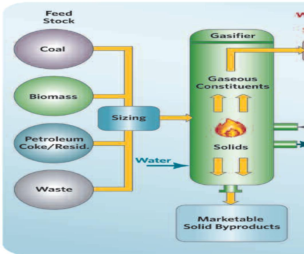
**Fig.2.** Overview of a gasifier for power production with relevant processes
