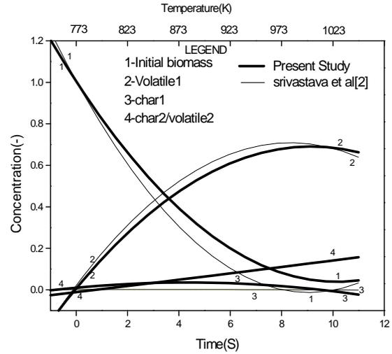
**Plot-1** Concentration Vs Time/Temperature under non-isothermal condition
