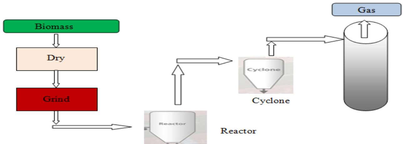
**Fig 1** Fuel gas generation using biomass
