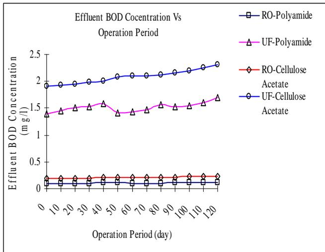
**Figure 2:** Conc. of BOD in the effluent of RO and UF system
