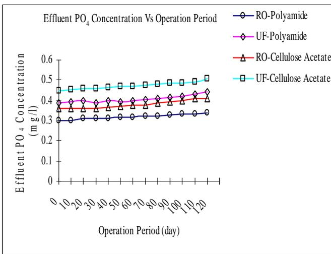
Figure 7: Conc. of PO<sub>4</sub> in the effluent of RO and UF system
