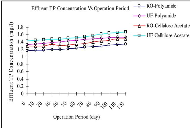
Figure 6: Conc. of TP in the effluent of RO and UF system
