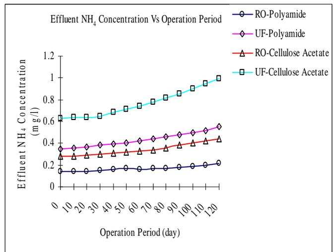
**Figure 5:** Conc. of NH<sub>4</sub> in the effluent of RO and UF system
