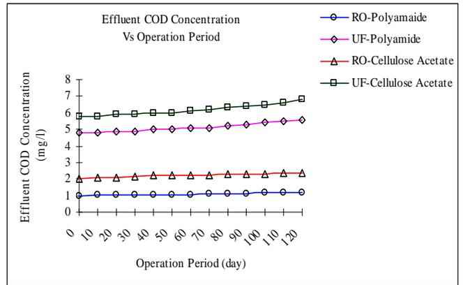
**Figure 3:** Conc. of COD in the effluent of RO and UF system
