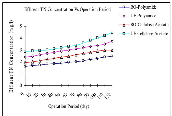
**Figure 4:** Conc. of TN in the effluent of RO and UF system
