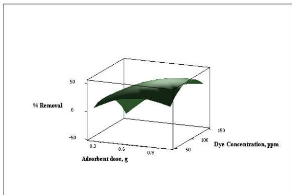
**Fig-4:** Surface plot of percentage removal of CV dye, Adsorbent dose and Dye concentration
