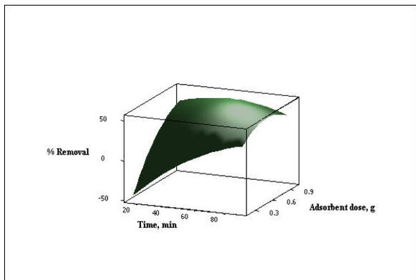
**Fig-3:** Surface plot of percentage removal of CV dye, Time and Adsorbent dose
