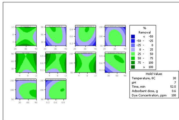
**Fig-12:** Contour plots of removal of CV dye
