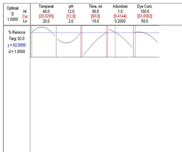
**Fig-13:** Response surface optimization plots for percentage removal of CV dye
