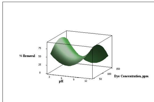
**Fig-6:** Surface plot of percentage removal of CV dye, Dye concentration and pH
