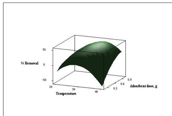
Fig-2: Surface plot of percentage removal of CV dye, Temperature and Adsorbent dose
