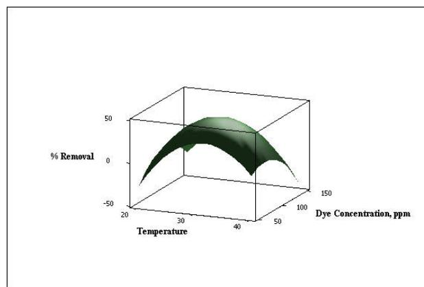
**Fig-7:** Surface plot of percentage removal of CV dye, Dye concentration and Temperature
