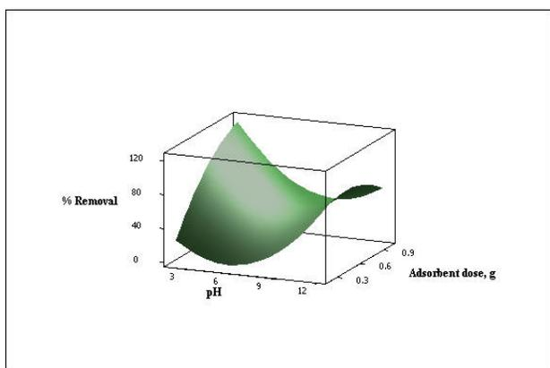
**Fig-5:** Surface plot of percentage removal of CV dye, Adsorbent dose and pH
