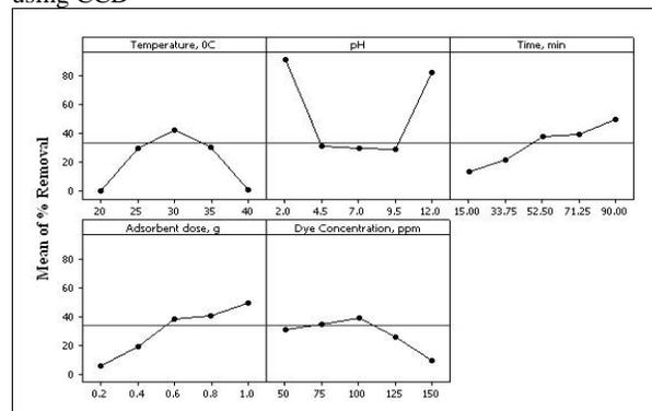
Fig-1: Main Effects plots of % Removal of CV Dye
