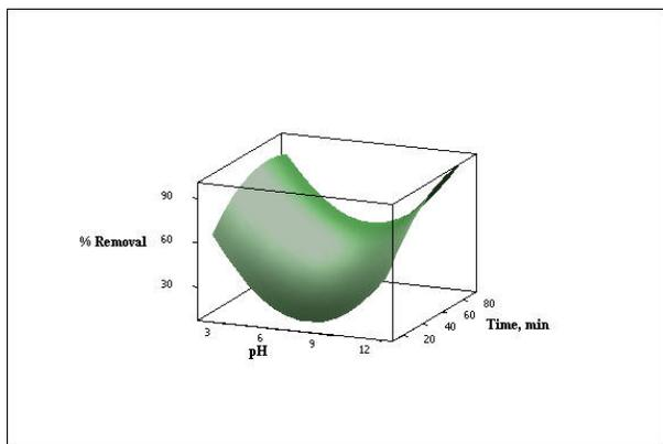
**Fig-10:** Surface plot of percentage removal of CV dye, pH and Time
