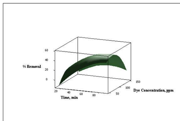
**Fig-8:** Surface plot of percentage removal of CV dye, Dye concentration and Time
