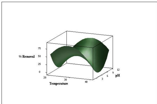
**Fig-9:** Surface plot of percentage removal of CV dye, Temperature and pH
