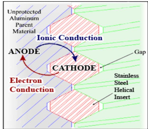
Figure 2: Galvanizing corrosion
