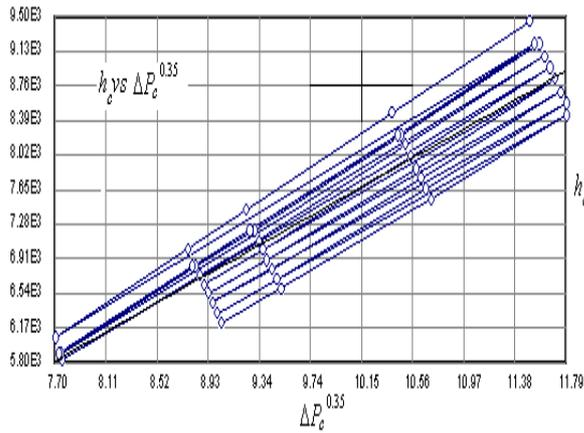
From the above [Figure 5, 6, 7 and 8] it is clear that, higher the pressure drop, greater the film heat transfer coefficient. The graphs of film heat transfer coefficient against Pressure drop were plotted using software polymath 5. The nature of line is straight and passes through the origin and slope is obtained as;
