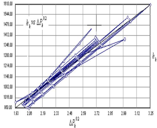
**Fig.6. Film heat transfer coefficient against Pressure drop For turbulent flow “hot water side”**
