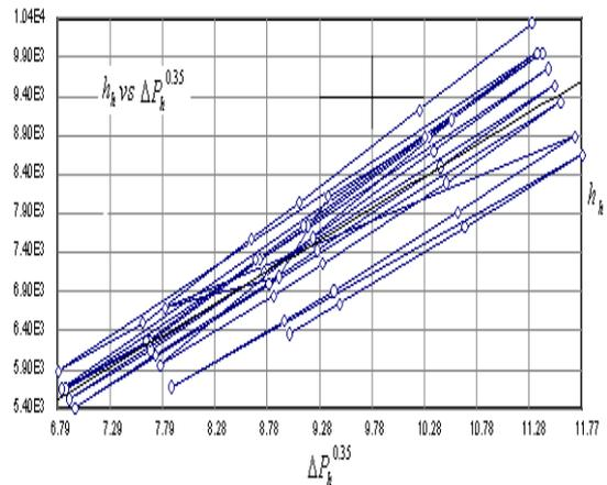
**Fig.7. Film heat transfer coefficient against Pressure drop For Laminar flow “Cold water side”**
