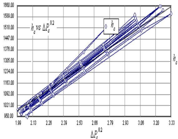
**Fig:8. Film heat transfer coefficient against Pressure drop For Turbulent flow “Cold water side”**
