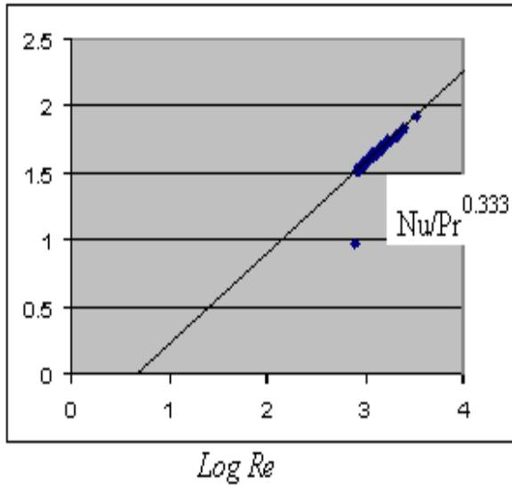
For the Reynolds number less than 800 the experimental data generates a straight line of slope approximately 0.333 which indicates the laminar flow conditions and the heat transfer correlation proposed as;
