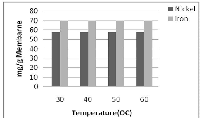
Fig. 4 : The effect of Temperature on removal capacity of Metal ions in Nafion 324
