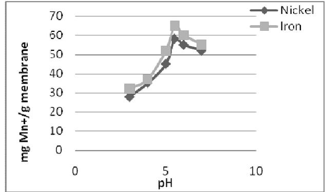
Fig. 3 : The effect of pH on removal capacity of Metal ions in Nafion 324
