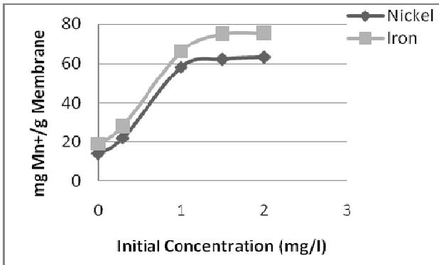
Fig. 2 : The effect of Initial Concentration on removal capacity of Metal ions in Nafion 324
