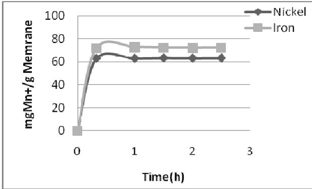
Fig. 1: Time required for the adsorption of Metal Ions in Nafion 324 membrane
