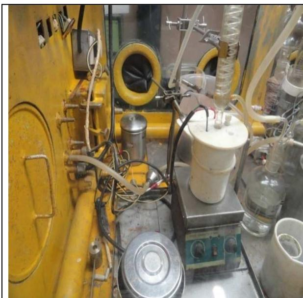
Fig. 1a. Apparatus used for dissolution of PuO<sub>2</sub>.
