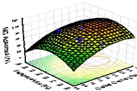
Figure 7: Effect of temperature and corn cob dosage on malachite green adsorption
