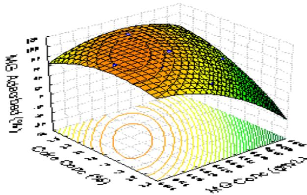
Figure 3: Effect of Malachite green and Coke dosage on dye adsorption
