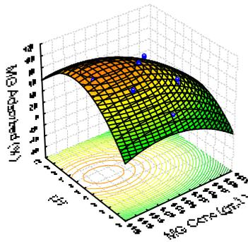
Figure 4: Effect of pH and Malachite green concentration on dye adsorption
