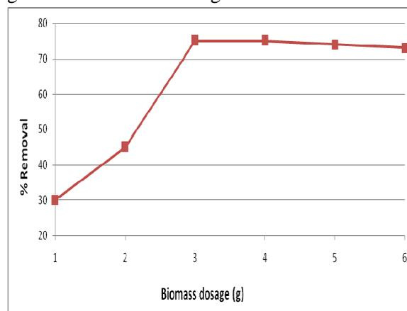
**Fig. 3:** Effect of adsorbent dosage on adsorption of iron on activated carbon of maize corncob (pH: 5.5, contact time: 120 min., iron concentration: 3 mg/L).
