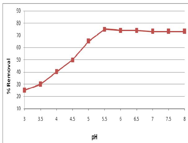
**Fig. 1:** Effect of pH on adsorption of iron on activated carbon of maize corncob (contact time: 120 min., iron concentration: 3 mg/L, adsorbent dosage: 3 g).
