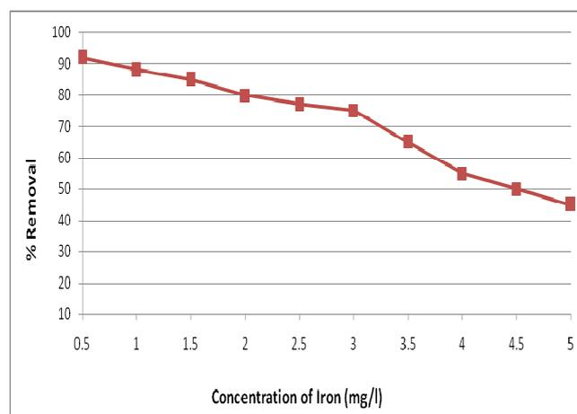
**Fig. 4:** Effect of iron concentration on adsorption on activated carbon of maize corncob (pH: 5.5, contact time: 120 min., 3 mg/L, adsorbent dosage: 3 g).
