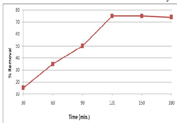
**Fig. 2:** Effect of contact time on adsorption of iron on activated carbon of maize corncob (pH: 5.5, iron concentration: 3 mg/L, adsorbent dosage: 3 g).
