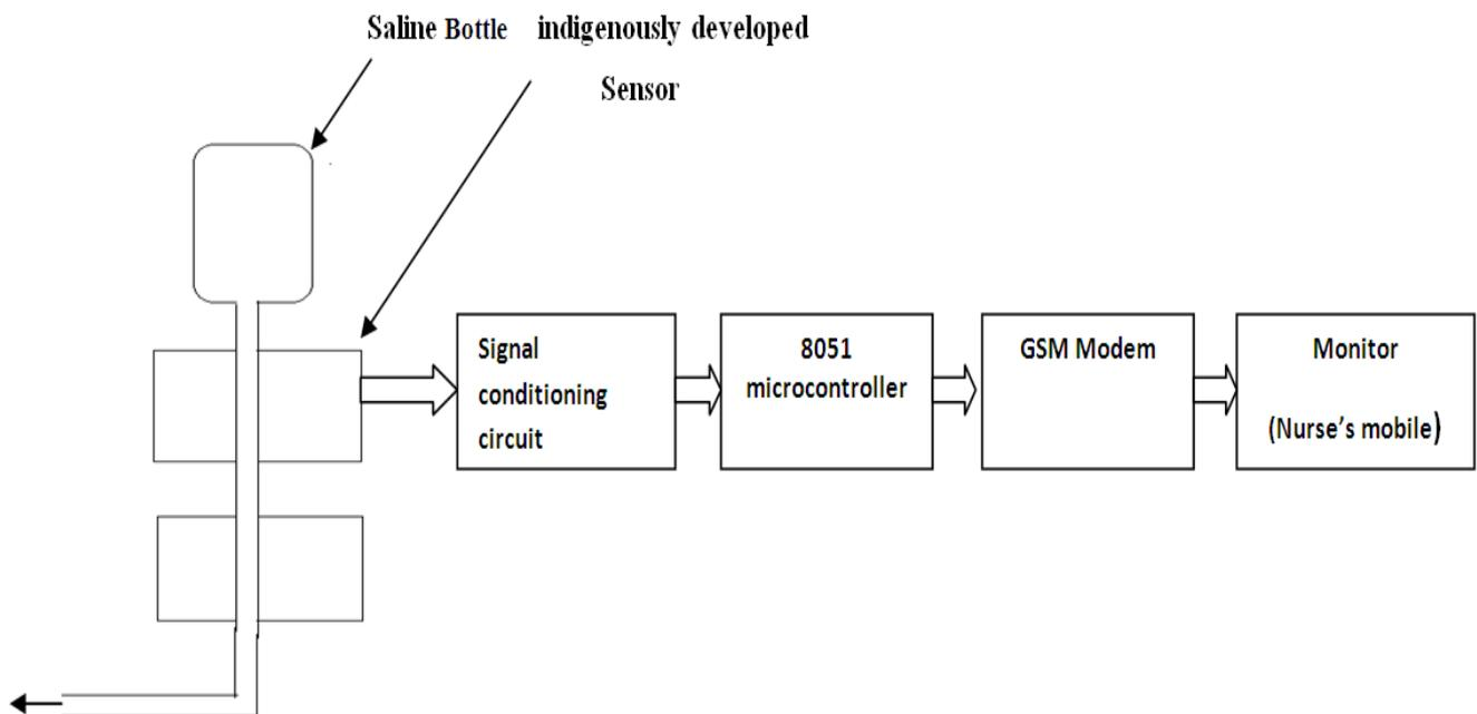
**Fig. 1: Block diagram of the saline monitoring system**
