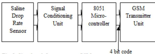
**Fig. 2: Signal path from sensor to GSM**
