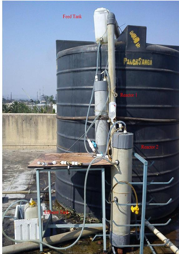
**Fig: 2.** Working Model of Two Stage UAPB Reactor
