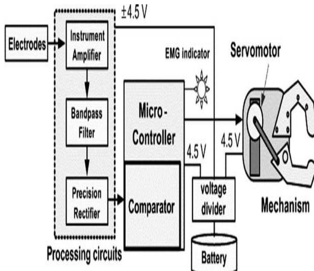
Fig. 4 Block presentation of prosthetic arm
