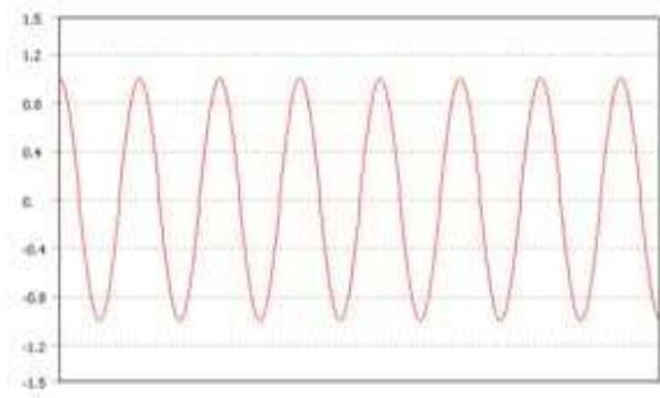
Figure 6. Constant amplitude fully reversed
