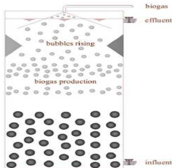
**Fig.2** Schematic diagram of UASB reactor
