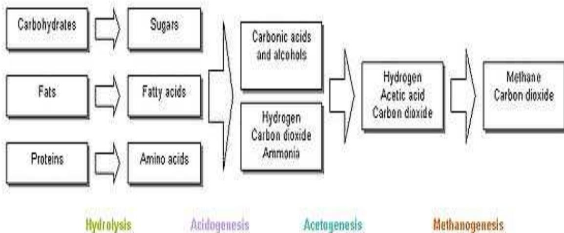
**Fig.1** UASB process stages
