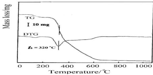
**Fig.1**DTA and TG curves of RH samples burning in air
