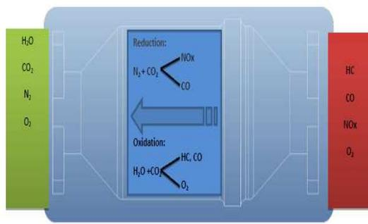
**Fig: 2.** Reaction occurring in catalytic converter
