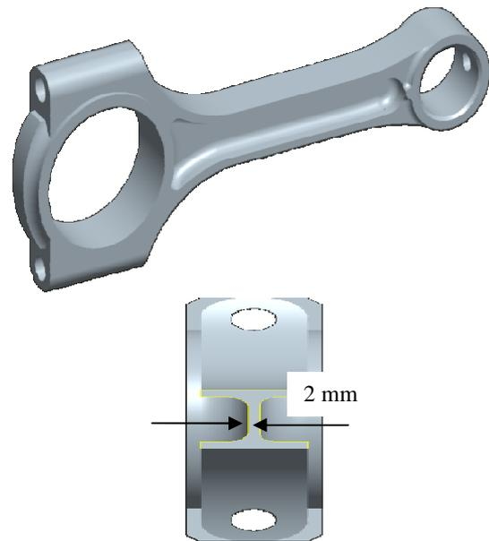
**Fig: 13.** Modified Connecting rod
