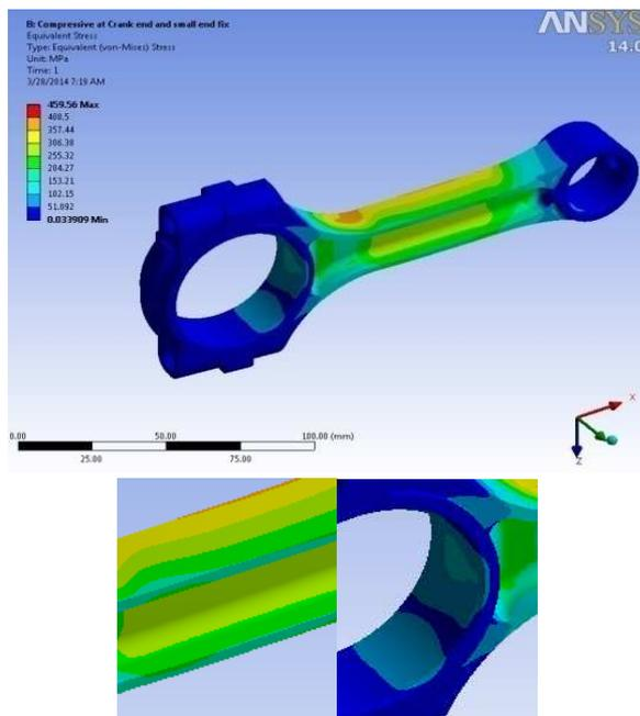
**Fig: 11.** Von Mises stresses with piston pin end fixed and static compressive load at the crank end.
