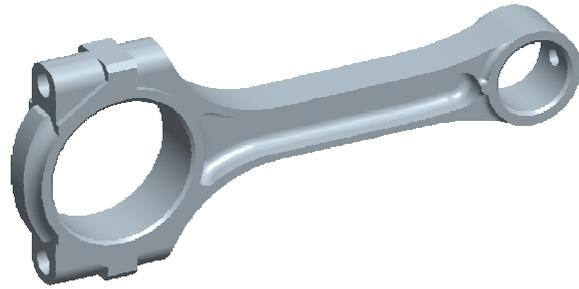
Fig. 1. 3D Solid model of Connecting rod.
