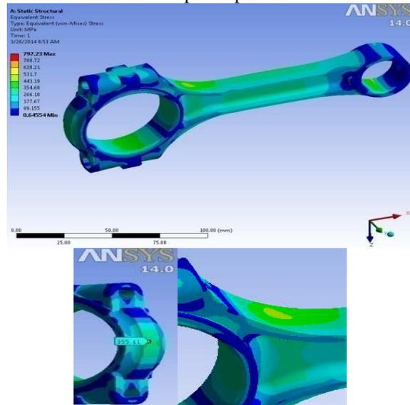
**Fig: 9.** Von Mises stresses with Crank end fixed and static tensile load at piston pin end.
