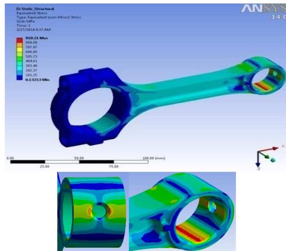
**Fig: 8.** Von Mises stresses with Crank end fixed and static tensile load at piston pin end.
