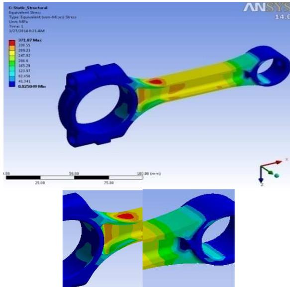
**Fig: 10.** Von Mises stresses with Crank end fixed and static compressive load at piston pin end.
