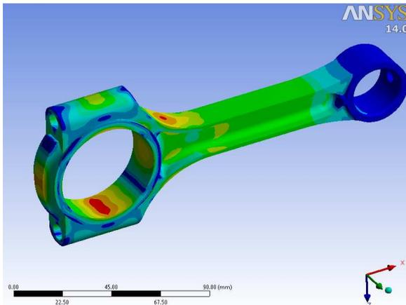
**Fig:14.** FEA of Modified Connecting rod.
