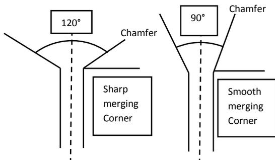
Fig. 3. Oil hole modification
