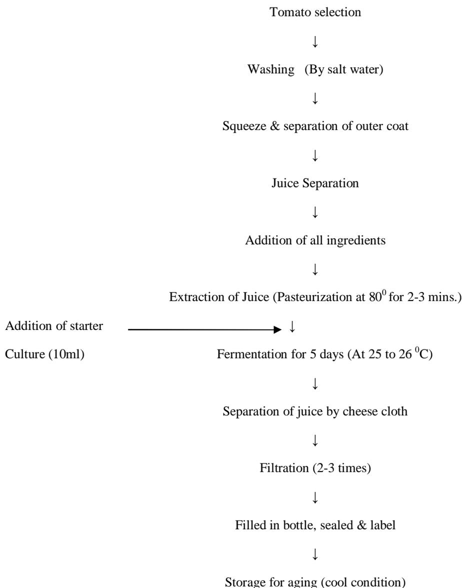
Fig. 1 Flow chart of alcohol preparation
