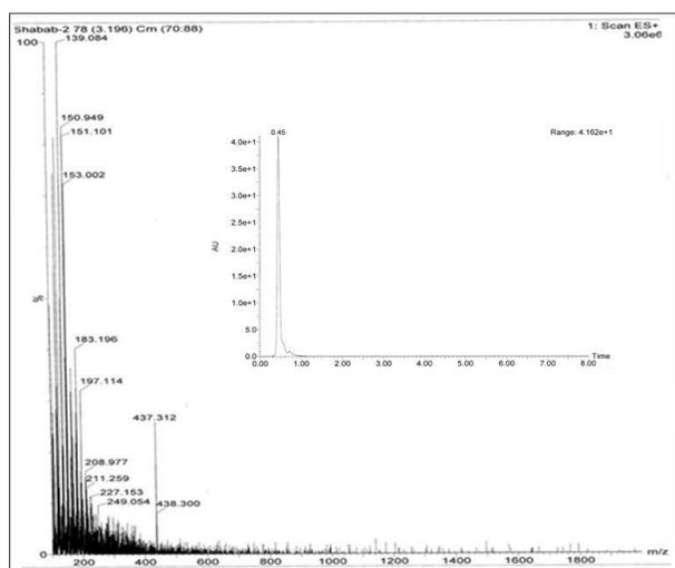
**Fig: 6.** Molecular mass of CPI. The purified CPI was analyzed for the determination of the Mr by electrospray ionization spectra (437.312 Da). (Inset)- Reverse phase-UPLC profile of CPI. 0.5 ml of the lyophilized CPI sample was loaded on rp-UPLC C18 column. The inhibitor was monitored on diode array detector.
