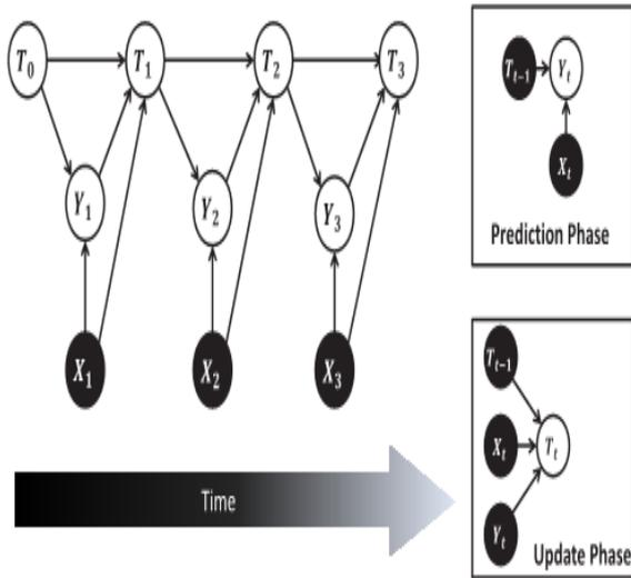
**Figure.2.**tracking processing line. It contains prediction phase and update phase at each time step. At the prediction phase, the algorithm predicts labels of the observation. At the update phase, the algorithm updates the tracking states.
