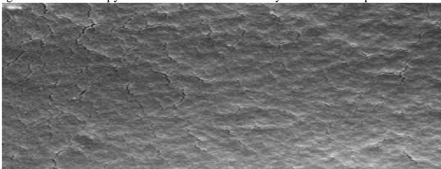
**Figure 4:** scanning electron microscopy of PMMA without nanocrystalline cellulose particles
