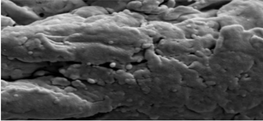
**Figure 1:** scanning electron microscopy of nanocrystalline cellulose particles
