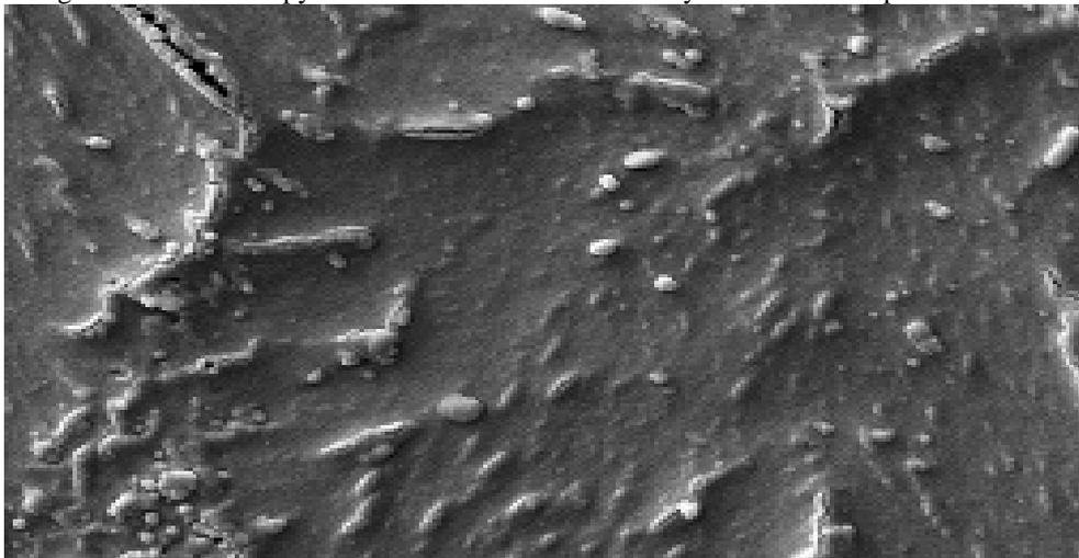
**Figure6:**scanning electron microscopy of PMMA with 5% wt nanocrystallin cellulose particle
