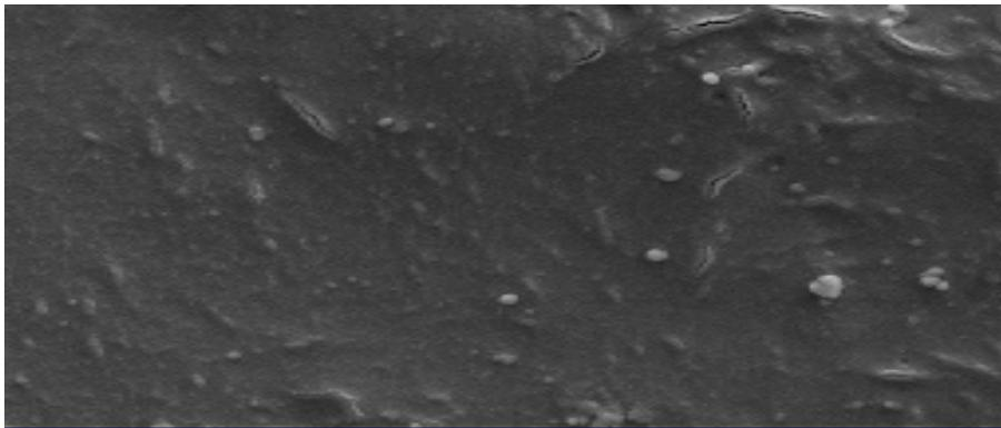
**Figure 3:** scanning electron microscopy of PMMA with 1% wt nanocrystalline cellulose particles
