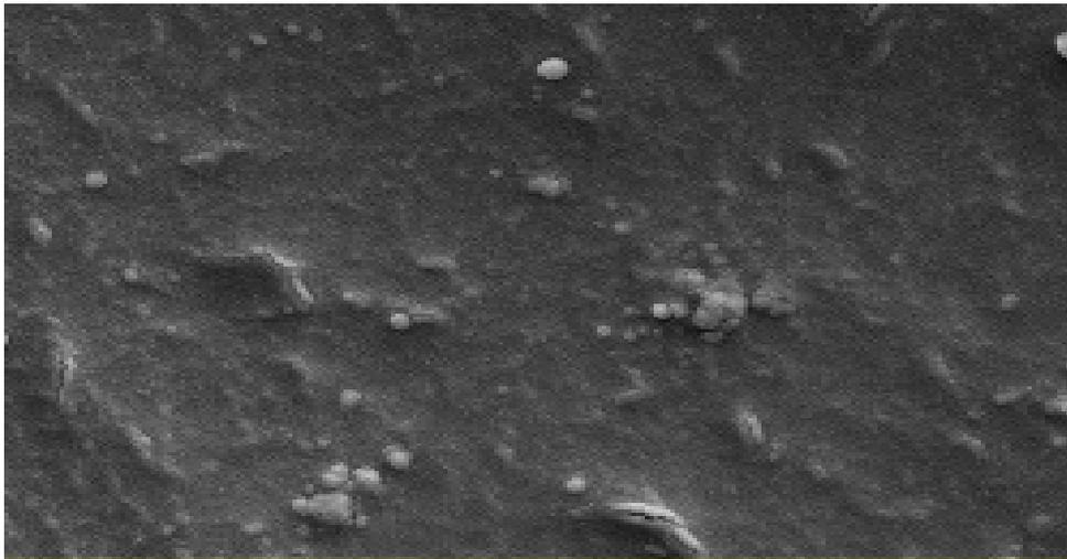
**Figure5:**scanning electron microscopy of PMMA with 2.5% wt nanocrystallin cellulose particle
