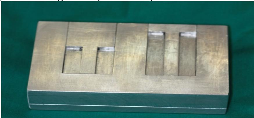
**Figure 2:** Aluminum mold
