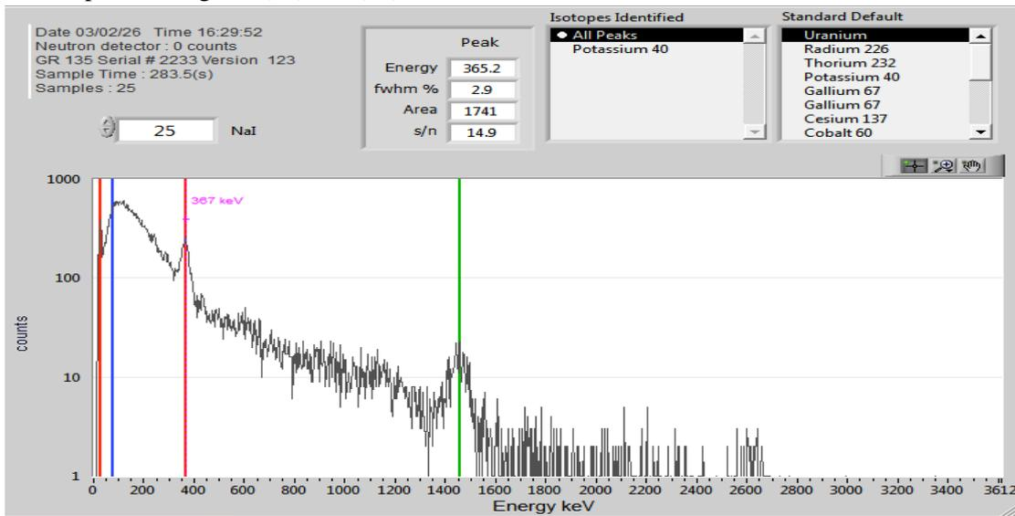
**Figure 13:** gamma spectrometer spectrum in detection for 300 seconds in the presence of 250 becquerel source in one thyroid lobe
