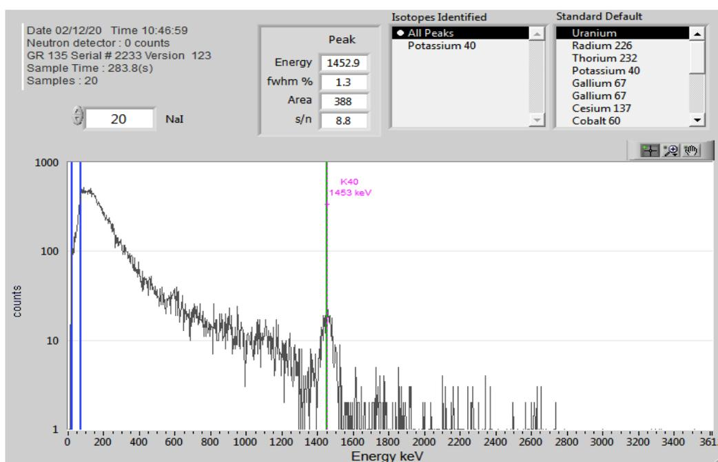
**Figure 12:** background radiation spectrum for 300 seconds of measurement
