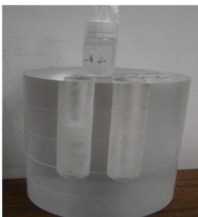
**Figure 1:** thyroid phantom made of Plexiglas with vials containing 131I- source
