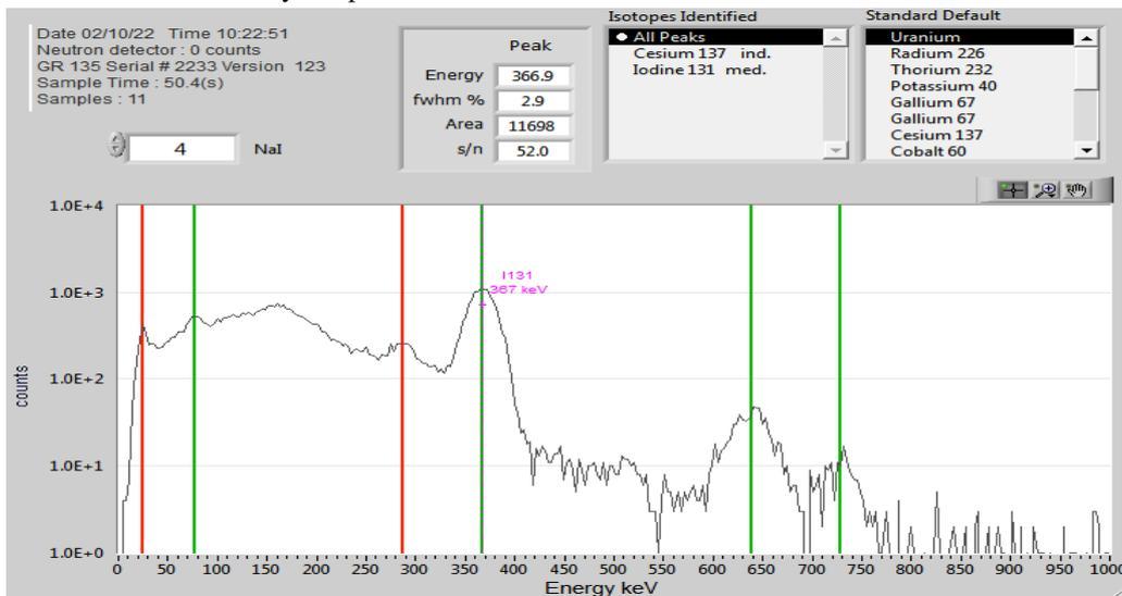
**Figure 3:** spectrum of gamma spectrometer in 55 seconds detection for distance of 5 cm and in presence of 129.5 kilo Becquerel source in one lobe of thyroid phantom
