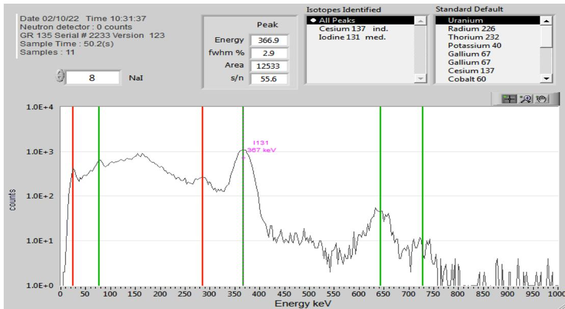
**Figure 9:** spectrum of gamma spectrometer in 55 seconds detection for distance of 15 cm and in presence of 351.5 kilo Becquerel source in two lobes of thyroid phantom
