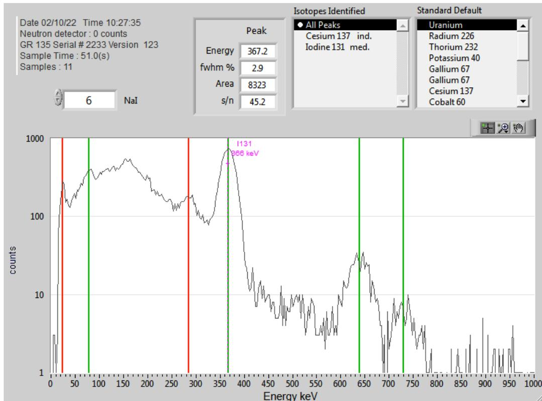
Figure 4: spectrum of gamma spectrometer in 55 seconds detection for distance of 10 cm and in presence of 129.5 kilo Becquerel source in one lobe of thyroid phantom
