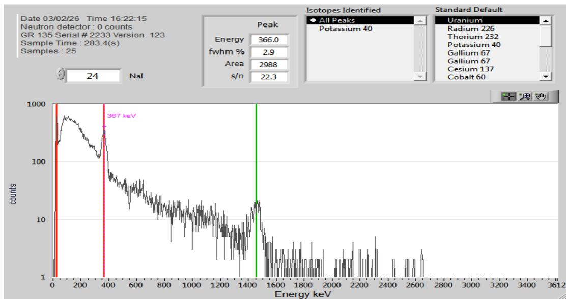
**Figure 14:** gamma spectrometer spectrum in detection for 300 seconds in the presence of 250 becquerel source out of the Thyroid phantom at the distance of 1 cm from the detector
