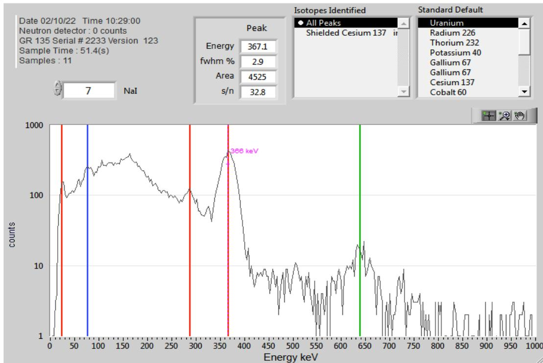
**Figure 5:** spectrum of gamma spectrometer in 55 seconds detection for distance of 15 cm and in presence of 129.5 kilo Becquerel source in one lobe of thyroid phantom
