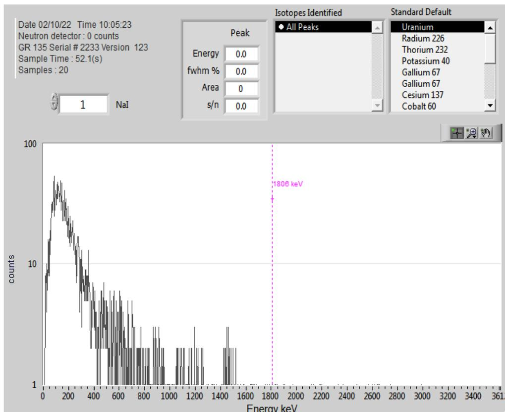
**Figure 11:** background radiation spectrum for 55 seconds of measurement
