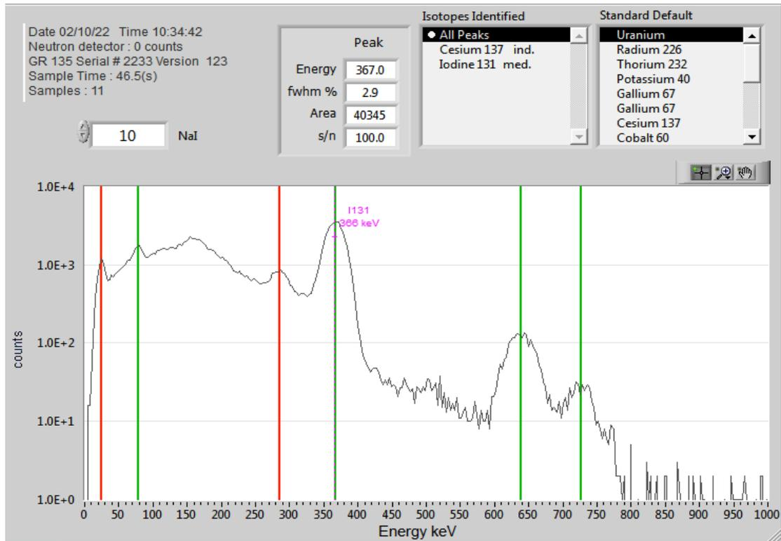
**Figure 7:** spectrum of gamma spectrometer in 55 seconds detection for distance of 5 cm and in presence of 351.5 kilo Becquerel source in two lobes of thyroid phantom
