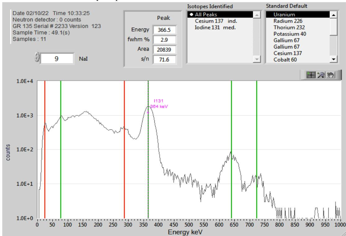
**Figure 8:** spectrum of gamma spectrometer in 55 seconds detection for distance of 10 cm and in presence of 351.5 kilo Becquerel source in two lobes of thyroid phantom
