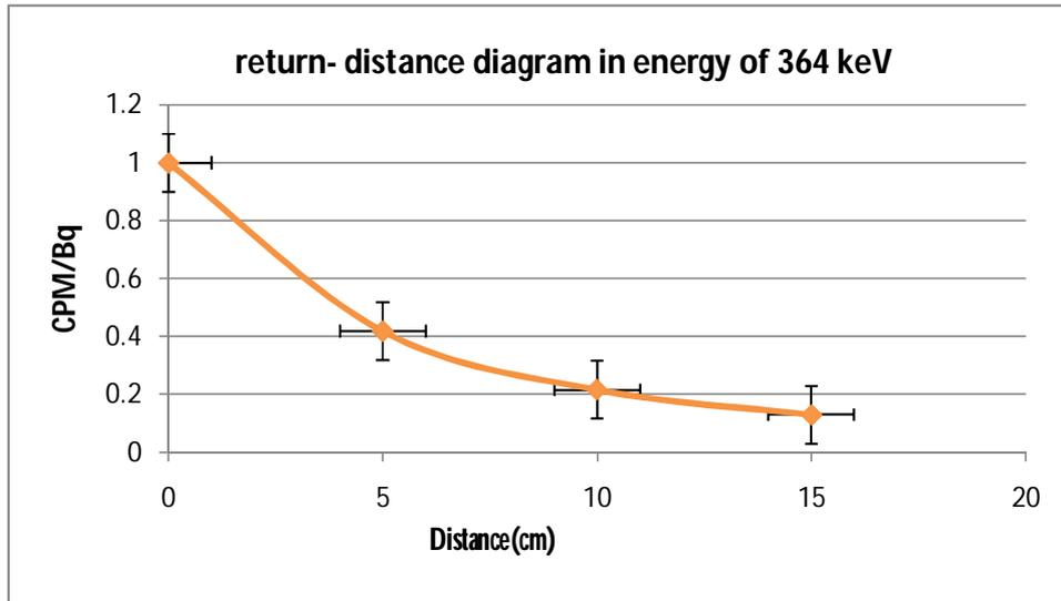
**Figure 10:** the dependency of normalized values of MDA in relation to the distance
