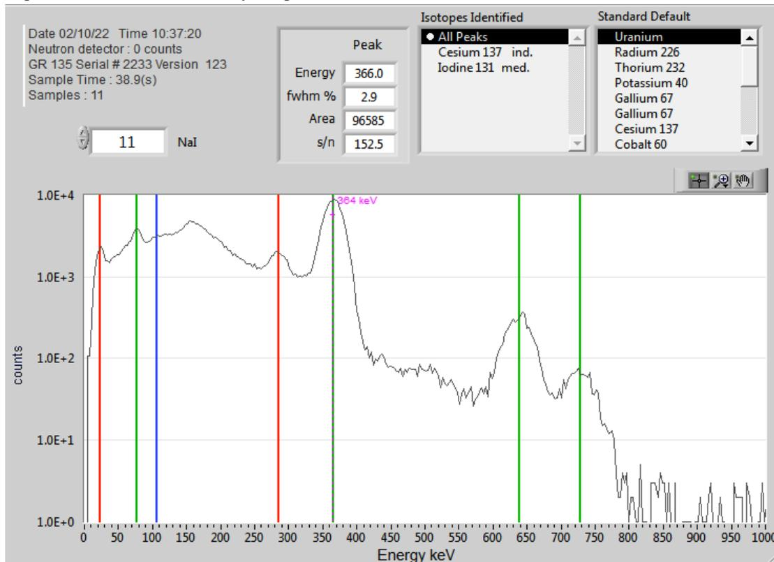
**Figure 6:** spectrum of gamma spectrometer in 55 seconds detection for distance of 0 cm and in presence of 351.5 kilo Becquerel source in two lobes of thyroid phantom
