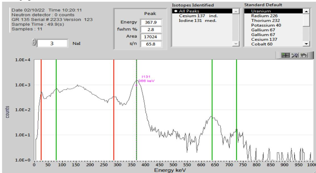
**Figure 2:** spectrum of gamma spectrometer in 55 seconds detection for distance of 0 cm and in presence of 129.5 kilo Becquerel source in one lobe of thyroid phantom
