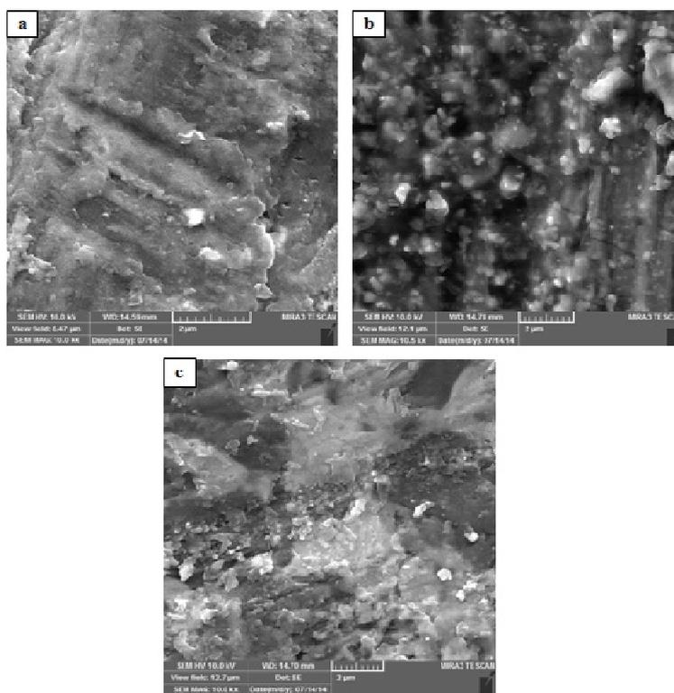
**Figure 2:** SEM image of sample with a) 0% b) 2% and c) 8% nano zirconia
