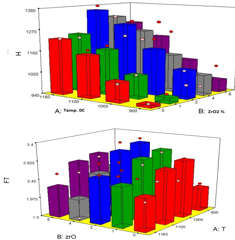
**Figure 1:** the effect of parameters on hardness (a) and Fracture toughness of samples
