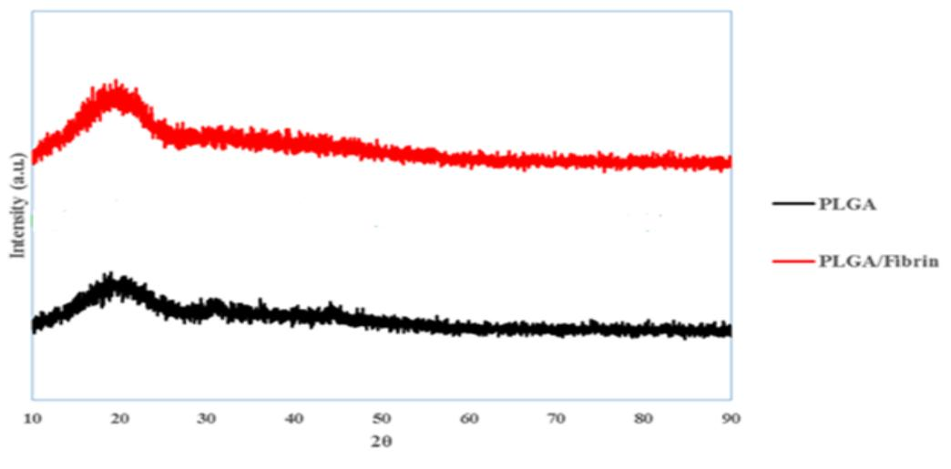
**Fig.1** The XRD patterns of the PLGA and the PLGA/fibrin scaffolds.
