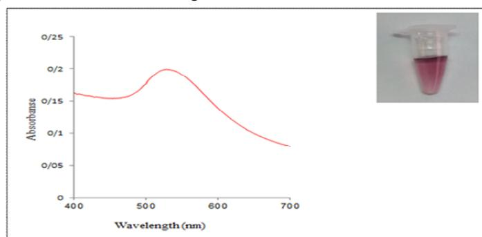
**Figure 5:** absorption spectrum of gold nanoparticles. As shown in the picture, the maximum absorption of gold nanoparticles occurred at the wavelength of 528 nm.
