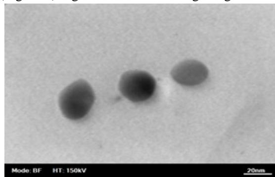
**Figure 4:** Image of gold nanoparticles synthesized by trisodium citrate taken by TEM with an enlargement of 140000, As is evident in the picture, all synthesized gold nanoparticles are spherical, yet no assembly is observed.
