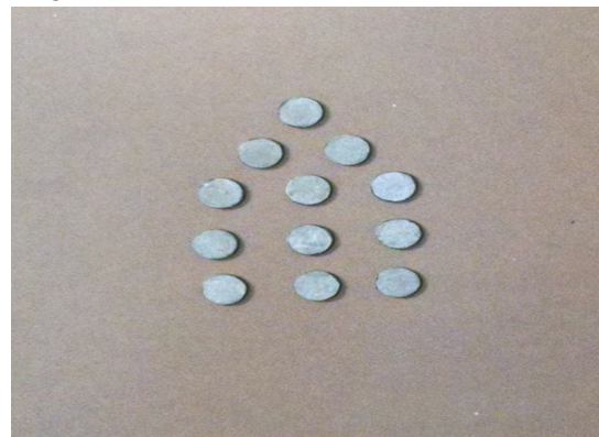
Fig.2: metal disks for feldspathic porcelain group
