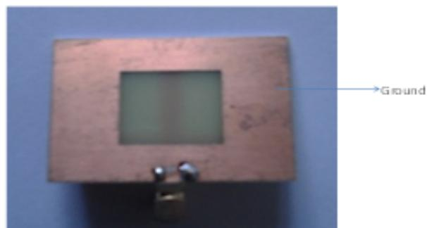
**Figure 4:** Inverted T shape Antenna (back view)
