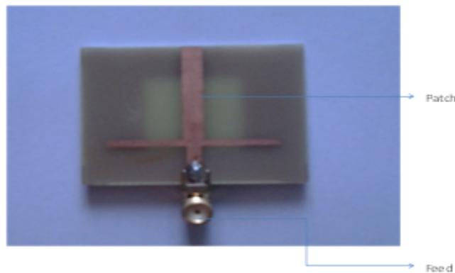
**Figure 3:** Inverted T shape antenna (front view)
