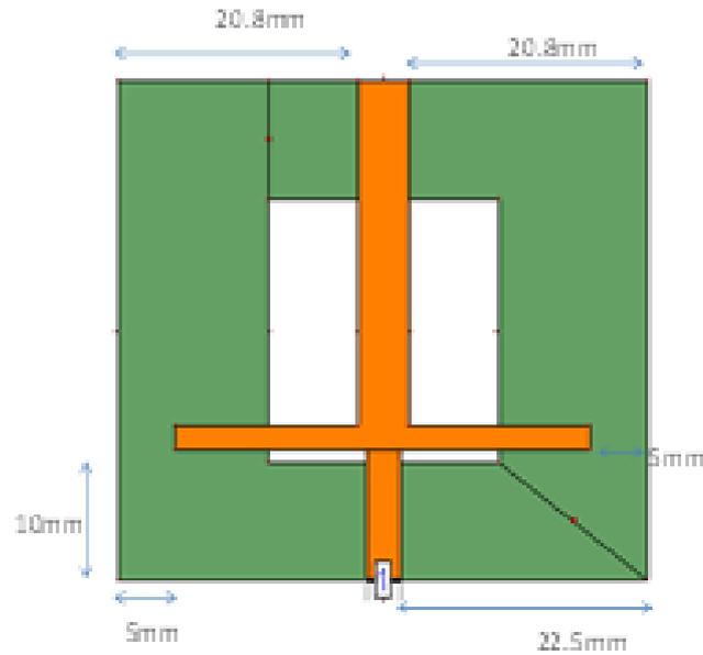
**Figure2:** Antenna Structure
