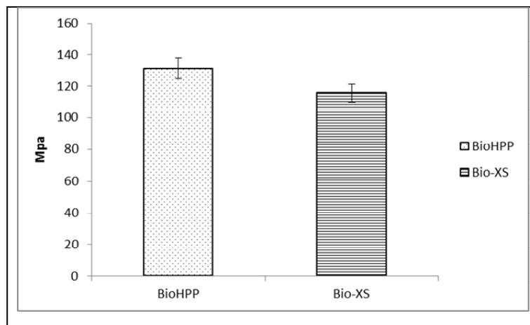
**Figure 2.** tensile strength of Bio-XS and Bio HPP thermoplastic resins
