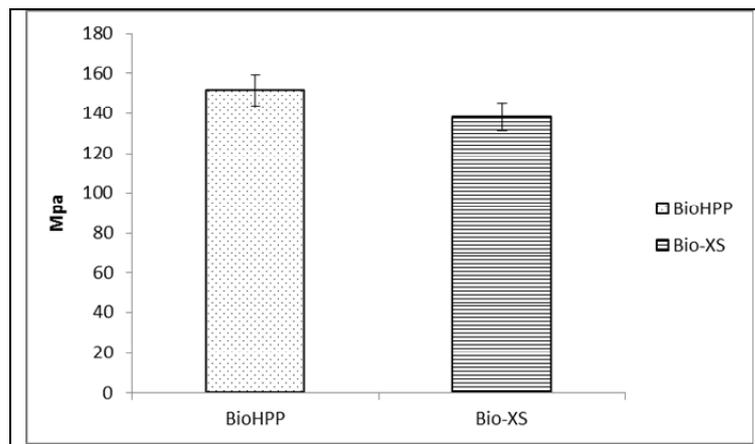
**Figure 1.** flexural strength of Bio-XS and Bio HPP thermoplastic resins
