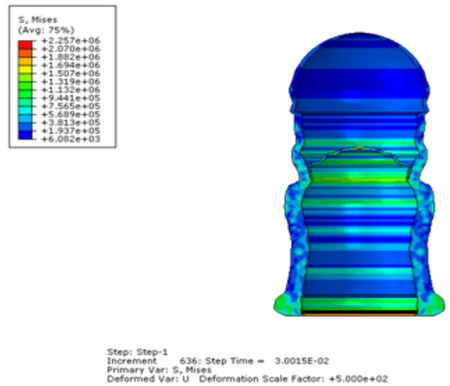
Fig.9. Damage of the load carrier in 0.03 seconds after the explosion began
