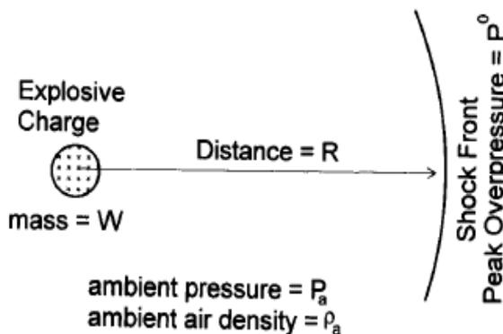
Fig.1. - Parameters effective in analyzing the explosive force
