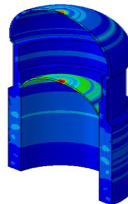
**Fig.7.** Von mises stress on dome
