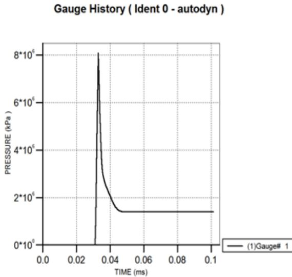
**Fig.3.** The pressure diagram applied to a point adhering to the explosive at the time of the explosion. As seen in the analytical relationship, the explosion wave is reduced by increasing the radius. This decrease in the power of the explosion wave is directly related to the cubic radius.
