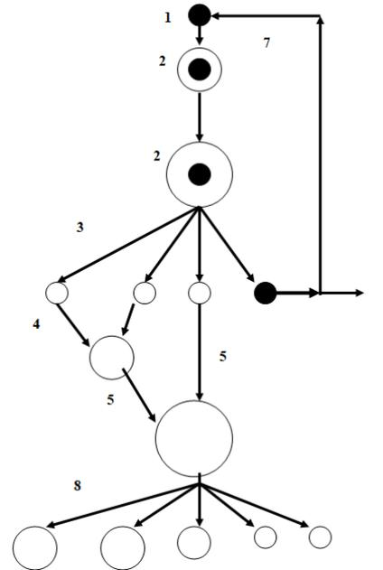
**Fig. 2.** Working hypothesis of the development of aggregates of anaerobically mixed culture. 1. Loading material. 2. Formation of biofilm on a carrier. 3. Separation of biofilm into smaller parts (fragments). 4. Adhesion of small parts (fragments); 5. Growth of aggregates. 6. Transfer of feed material from the reactor. 7. Return of the load to the biofilm formation process. 8. Fragmentation of large particles.
