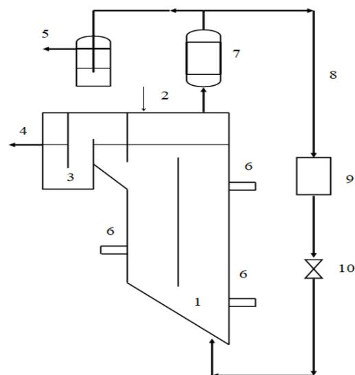
**Fig. 1.** Schematic diagram of an anaerobic reactor.
