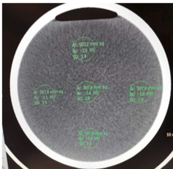
**Figure 3.** Field uniformity obtained from water phantom scan by Philips 64 slices scanner
